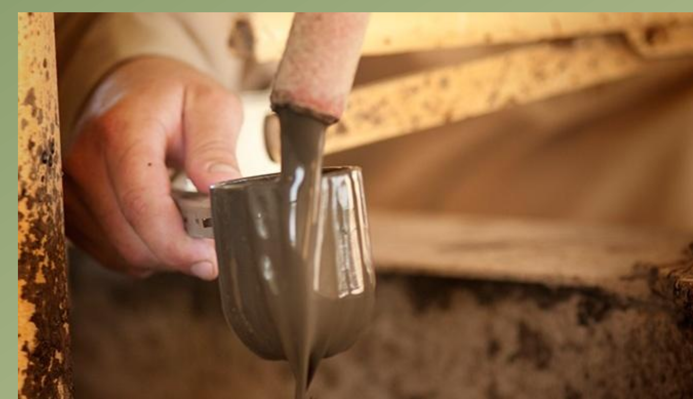
Pic (1):drilling mud
